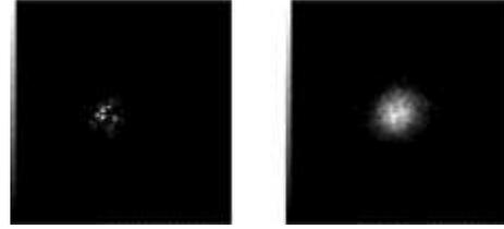
**Figure 1 - Simulation results showing a short (left) and long (right) exposure of a star through turbulence. Turbulence strength was estimated with  $D/r_0 = 10$ . These results you can ‘freeze’ the turbulence and get a clearer image. However, the short exposure image on the left, is speckled which result from the interference of light from many coherent patches, each with a diameter of about  $r_0$ , distributed over the full aperture of the telescope. [13]**
