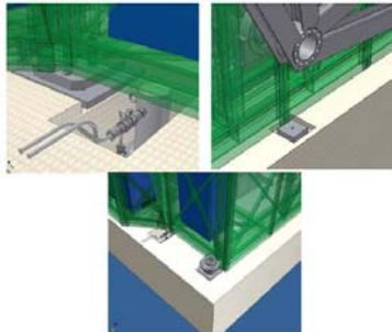
Figure 7. Close up of the interface foundation interfaces. (Courtesy of EIE).
