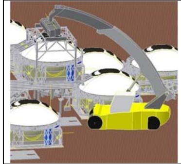
Figure 12. Cartoon of the reachstacker transporting the enclosure with telescope inside. (Courtesy of EIE).
