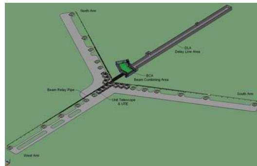
Figure 2 - Schematic plan view of the MROI Interferometer showing the general equilateral “Y” arrangement of the array arms with the proposed locations of the 28 telescope stations. The Beam Combining Facility, into which light from the individual telescopes will be directed, is the grey shaded structure running east from the vertex of the array.
