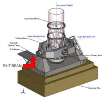
Figure 1 - The 1.4m aperture MROI elevation-over-elevation unit telescopes. (Courtesy of AMOS)
