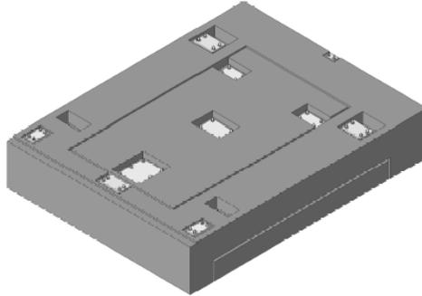
Figure 5. Station foundation showing the enclosure foundation seated over the UTM foundation but separated from each other by a vibration isolating membrane. (Courtesy of EIE).
