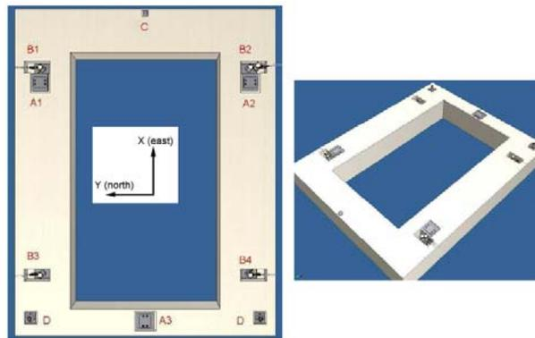
Figure 6. Enclosure foundation showing interface points: A = the fixing plates, B = relocation jacks, C = grounding plate, D = alignment plates. (Courtesy of EIE).
