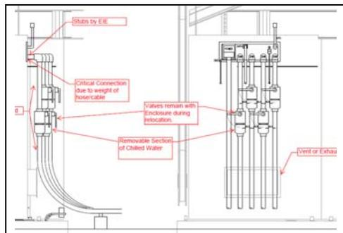
Figure 11. Detail of the Utility Interface Plate. (Courtesy of M3).
