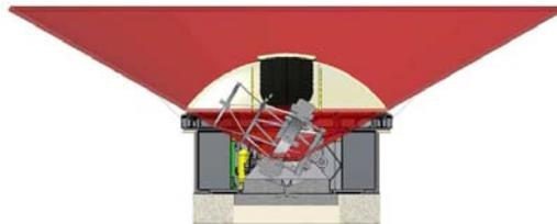
Figure 9. Light Path Boundary Cone with UTM detail at altitude angle of 30° (Courtesy of EIE).
